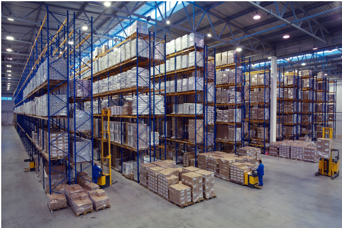
Figure 1: Typical high-bay warehouse aisles with long runs and high fire load
